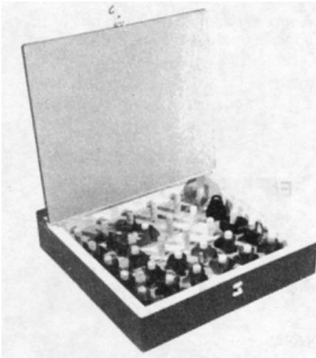
**Figure 9-10.** This shaper cutter storage case hold up to 30 three-lip shaper cutters.
